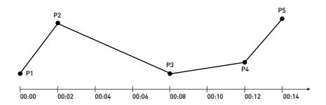
The fixture moves on the direct way from one position to the next, changing its movement direction at each point. If you want a smoother movement instead, you can select the option "Smooth movements".
