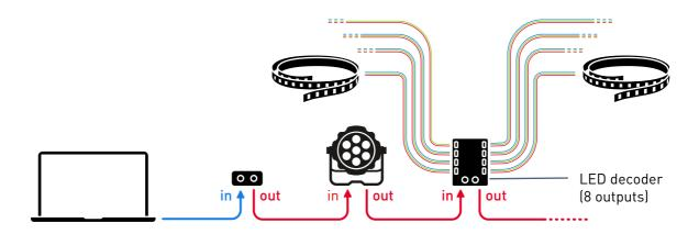
Some more advanced fixtures have RJ45 (Ethernet) ports and can receive data directly from the computer or through an Ethernet router or switch using network protocols like Art-Net or Streaming ACN (sACN or ANSI E1.31). Most of these fixtures also have an RJ45 out port so they can be daisy-chained.
