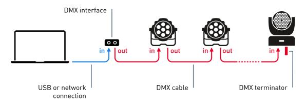
Each daisy chain of fixtures forms a **DMX universe** which operates up to 512 channels. For many installations a single universes is sufficient, but Lightkey can control up to 16 full universes or 8192 channels. Network interfaces with two, four, eight or more outputs let you send DMX to multiple separate DMX chains.
