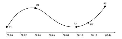
Lightkey will adjust the time at which each position is reached so that the fixture moves at (approximately) constant speed (ignoring the individual hold/fade times). The total time for moving through the sequence is still the same (that is, it is determined by the total hold and fade times).
