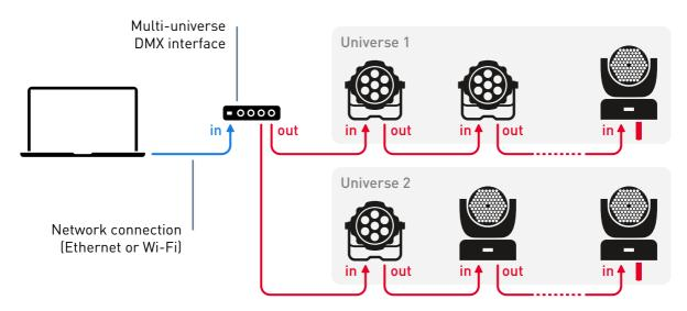
Another way to output multiple universes is to use multiple DMX interfaces. However, there are various limitations which are explained in chapter 14, DMX output and input. For example, Lightkey can only control a single USB interface and a single Art-Net node. Using a single DMX interface is the preferred way to output multiple universes.
