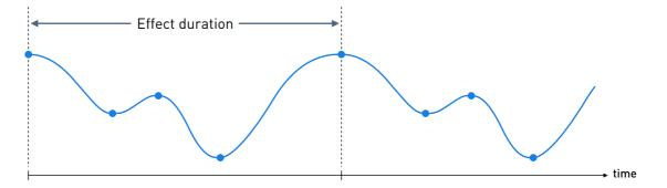
• Line: The fixture moves on the direct way from one control point to the next, changing its movement direction at each control point. The time for moving from one point to the next depends on the distance between the points.
