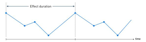
• **Points:** The fixture moves instantly from one control point to the next, with maximum speed. It remains at each control point for an equal time. (This is often used together with the "Blackout during pan/tilt movement" feature of many moving lights.)
