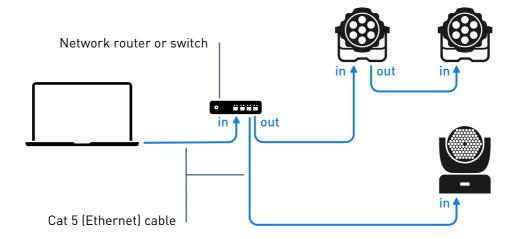
Some network-enabled fixtures can also route the Art-Net or sACN input to their XLR out port, so you can connect more fixtures with DMX cables. The exact capabilities depend on the fixture; please refer to the fixture documentation for details.
