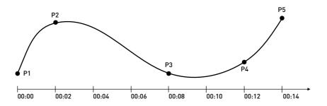
Lightkey will calculate a curve which passes all five fixture positions at the times determined by the steps' hold and fade times. For example, the time it takes to move from P1 to P2 is the sum of the first step's hold and fade times (with this option there is no longer a difference between hold and fade time).
